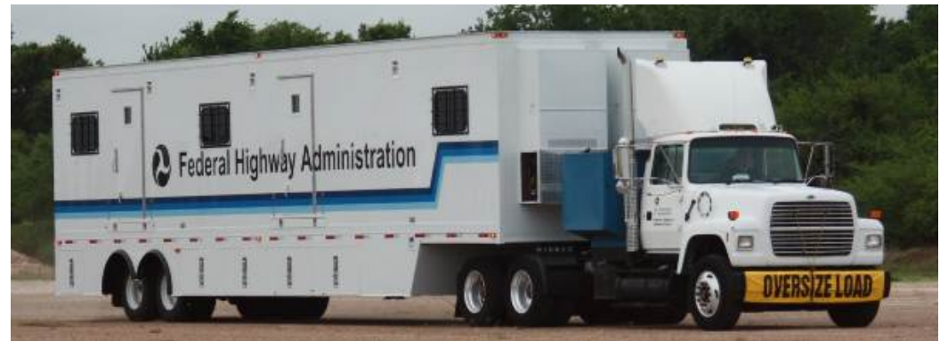
Mobile Asphalt Testing Trailer
