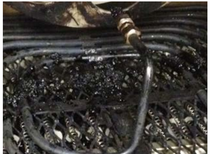
Asphalt Binder dripped onto Heating Elements inside RTFO Oven
